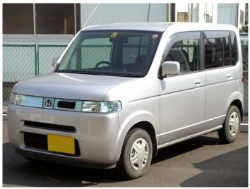
Yet another Kei car, the That's is enough to send your grammar checker crazy while you're typing its name. This tiny, but tall car had a three-cylinder, 656cc engine (naturally aspirated or turbocharged) and was manufactured for the Japanese market between 2002 and 2007. As the story goes, Honda hoped the name would become so appealing that onlookers would shout 'That's it!' when one went by.
