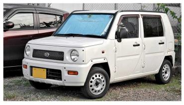
Although this Kei car – the smallest category of Japanese road-legal motor vehicles – had a strange name, the 658cc petrol Naked was oddly appealing and practical. Built between 1999 and 2004, the Naked had Jeep-like styling, an optional four-wheel-drive system and a rugged look with exposed bolts and hinges. Inside, its plastic
