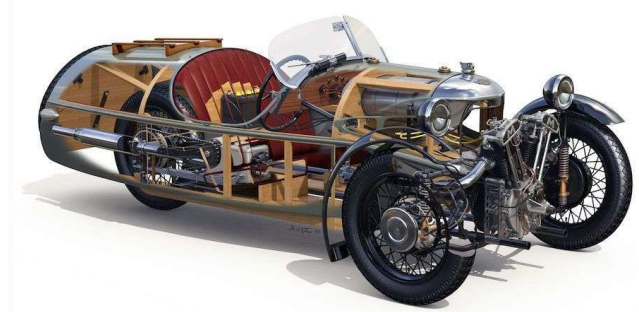
Morgan three-wheeler cutaway
