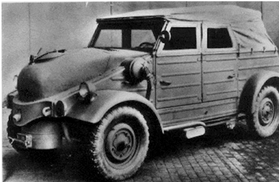
VW Kübelwagen with gas-producer mounted in front of the axle.
