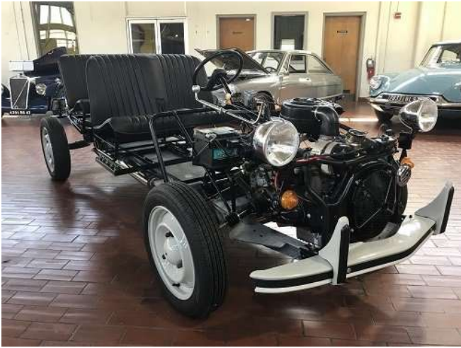
Citroen 2CV Bare Chassis - Note that the suspension units connect the front and rear wheels together and run horizontally under the vehicle.
