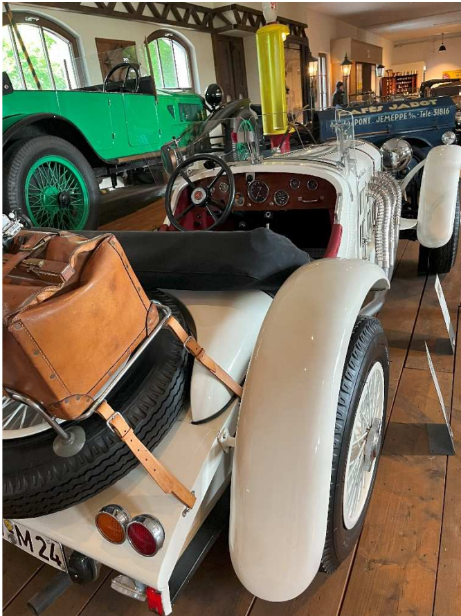
Mercedes SSK – Built 1928 to 1932 6cyl. 6800ccm. 130hp, V_{\max} = 200\text{km/h}
