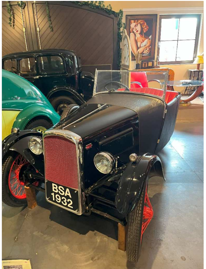
BSA – Three-Wheeler. Year 1932, 2cyl. 1100ccm, 27hp, V_{\max} = 100\text{km/h}
