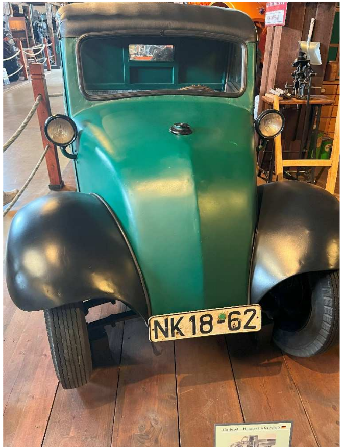
Gutbrod Hermes Transporter – 1 cyl. 194 ccm, 7hp, V_{\max} 40 km/h
