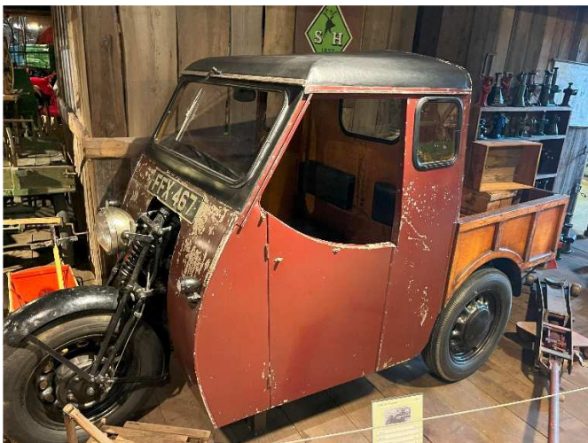
Reliant Regent – Year 1950, 747 ccm 18 hp. Built from motorcycle parts and an Austin Seven Motor. V_{\max} 50 km/h
