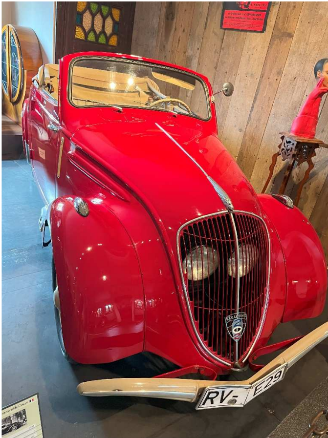
Peugeot 202 Convertible – Year 1938 4cyl. 1133ccm, 30hp, V_{\max} = 100\text{km/h} . The car was extremely economical @ 7.4l/100km fuel consumption
