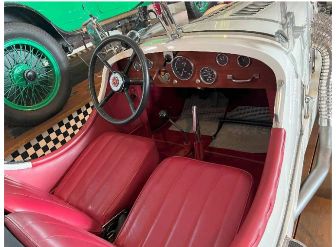
Mercedes SSK – Built 1928 to 1932 6cyl. 6800ccm. 130hp, V_{\max} = 200\text{km/h}
