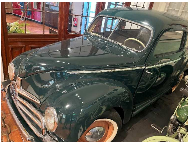
Ford Taunus – Year 1951, 4 cyl. 1200ccm, 34hp, V max 105km/h. The car was already designed and presented in 1939, but WW2 delayed production until 1949
