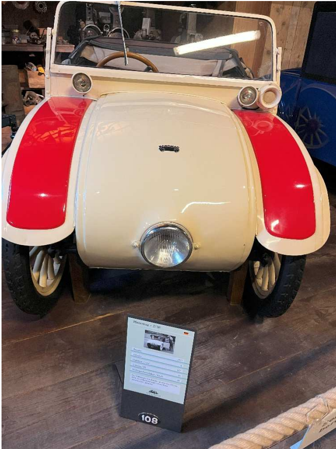
Hanomag – Germany Year 1927, 1 cyl. 500ccm 10hp, V_{\max} = 60\text{km/h}
