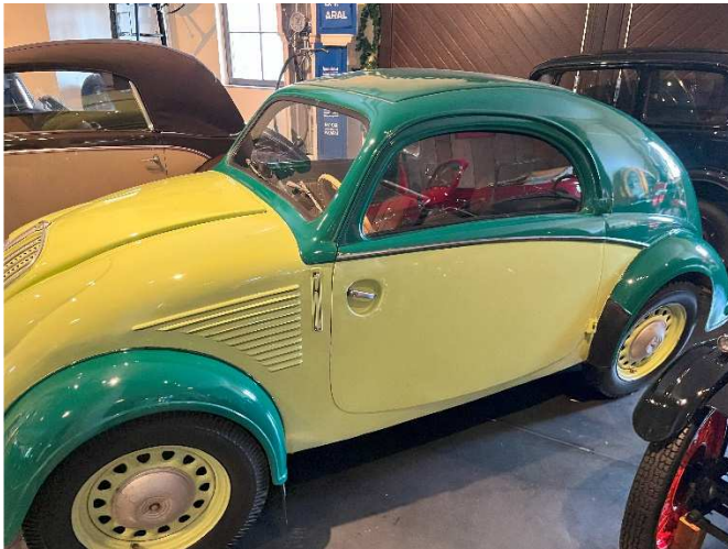
Steyr - 50 Baby - Austria, Year 1957, 4cyl. 960ccm, 22hp, Vmax= 90km/h. It was known as the Austrian "Beetle". It had a steel sunroof, a novum at the time
